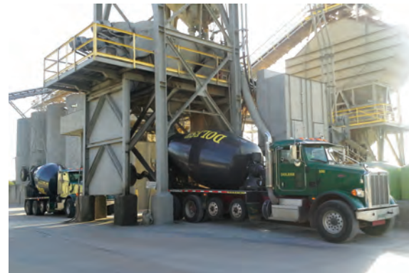
Figure 1-2. Ready mixed concrete is conveniently delivered to jobsites in trucks with revolving drums.
