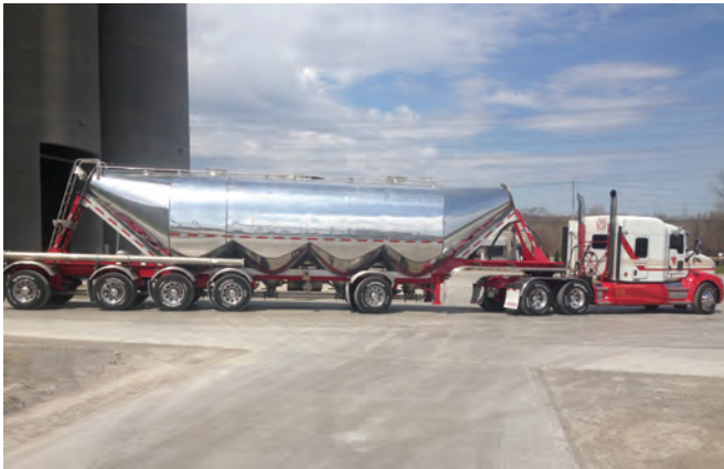
Figure 1-6. The majority of cement is shipped to concrete producers in cement haulers (tankers).
